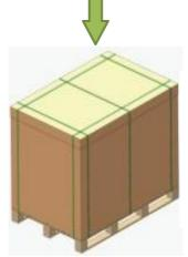
2. Cut off the packing straps of the single pallet, then remove the isolated wood (or plastic wrap) and the carton cover.
