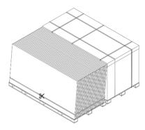
4. Stand on both sides of the short side of the module and slowly lean the module towards the support, and when the module is completely leaning on the support, cut the remaining bottom horizontal packing strap on the short side; finally, remove all modules sequentially from the outer one.
