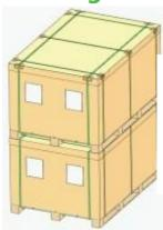
1. Cut off straps within the two pallets, and use a forklift to separate the two pallets.
