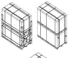
Remove the wrapping film around the box, then cut the cross-packing straps and remove the exterior wooden protector.
