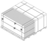
3. Remove the top cover of the box, and then remove the carton by lifting it. Two persons hold the modules to prevent them from tipping over. The other person cuts the top 2 horizontal straps and the 2 vertical straps of the modules, retaining the bottom horizontal strap.
